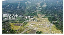
In October 2013, mudslides with driftwood occurred in several areas including Okanasawa, due to heavy rains caused by an approaching typhoon, resulting in extensive damage. Under such circumstances, these erosion control facilities were effective in mitigating the damage, by trapping large amounts of driftwood and large rocks upstream and damming the sediment downstream.
